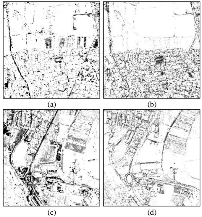
Fig. 2. RN noise maps obtained with the standard (left) and the proposed (right) approach on: (a), (b) the first dataset; and (c), (d) the second dataset.
