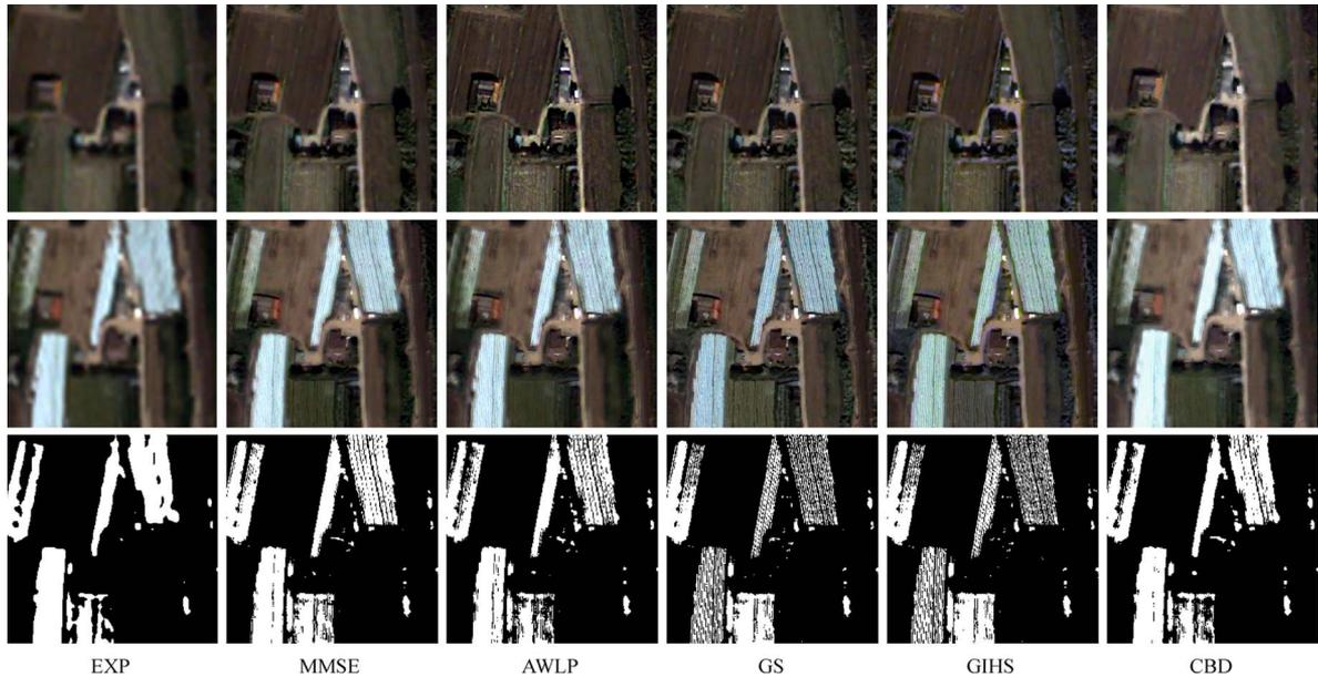
Fig. 2. True-color composite of  $256 \times 256$  details of 0.7-m QB data acquired on October 2005 (first row) and July 2006 (second row) for the upscaled and five pansharpened images. CD maps obtained for the upscaled and the five pansharpened multitemporal pairs at 0.7 m of resolution (third row).
