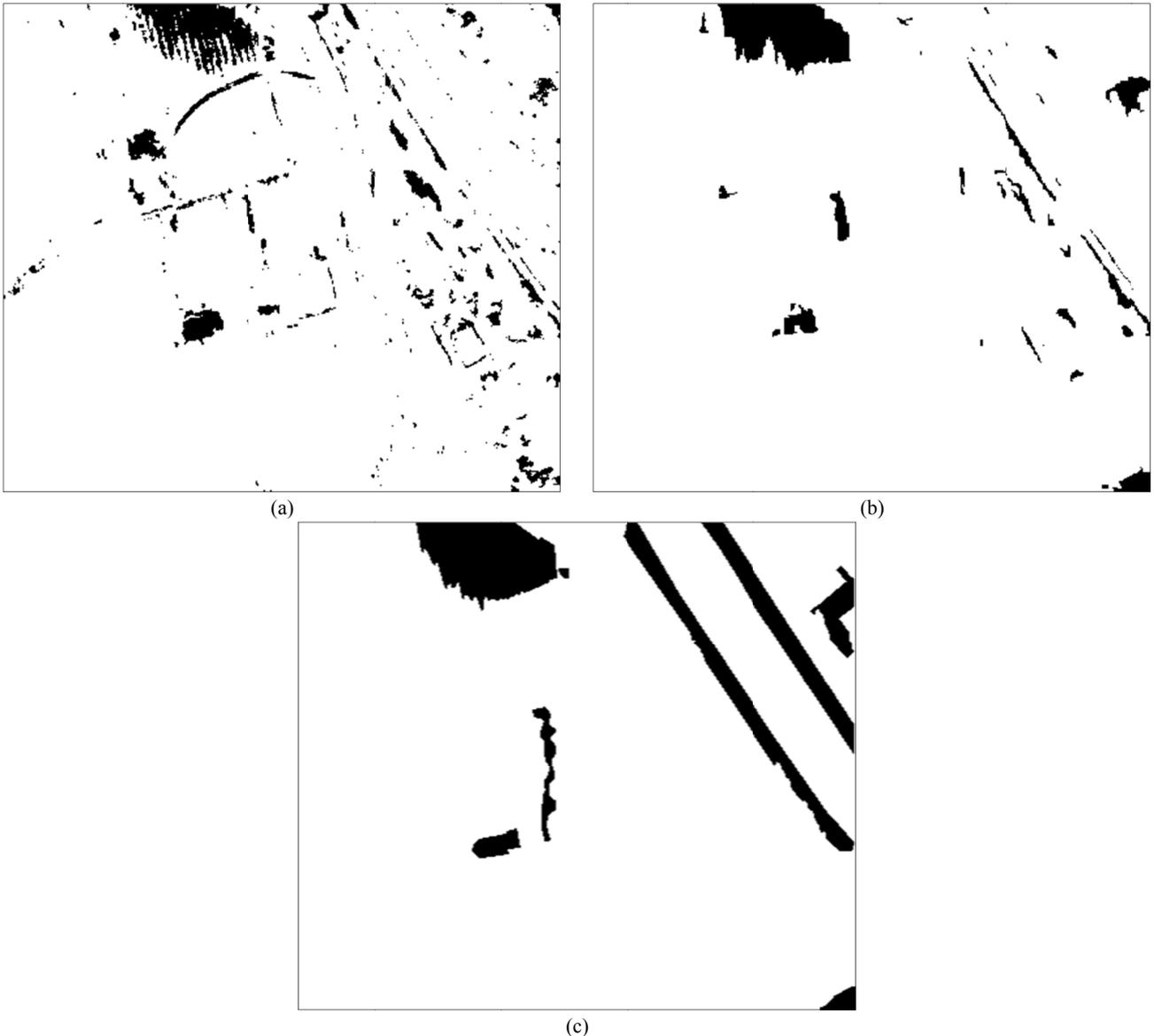
Figure 14 Change-detection maps obtained by (a) the pixel based Change Vector Analysis, and (b) the proposed method. Reference map of changes of interest (black color).
