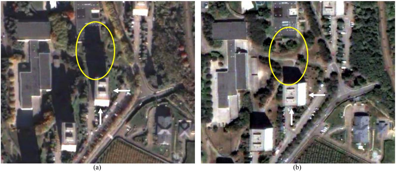
**Figure 2** Multitemporal image pair showing the effect of acquisition conditions in terms of acquisition sensor view angle and sun incidence angle. Images were taken from the QuickBird VHR sensor over the city of Trento, Italy, in: (a) October 2005 and (b) July 2006.
