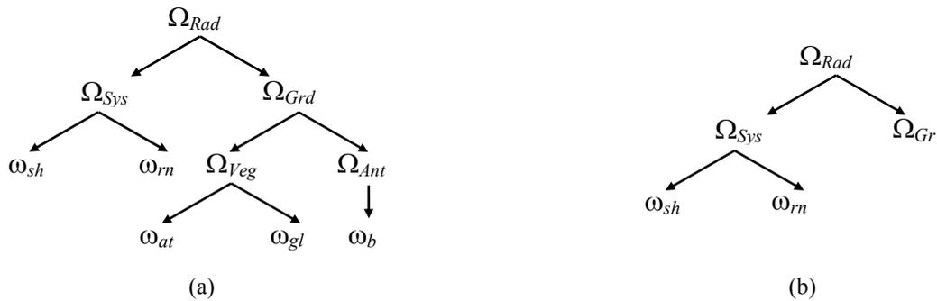
**Figure 10. Tree of radiometric changes for the considered problem: (a) complete tree describing all radiometric changes; and (b) pruned tree that describes the radiometric changes relevant to the final goal of the specific change detection problem.**
