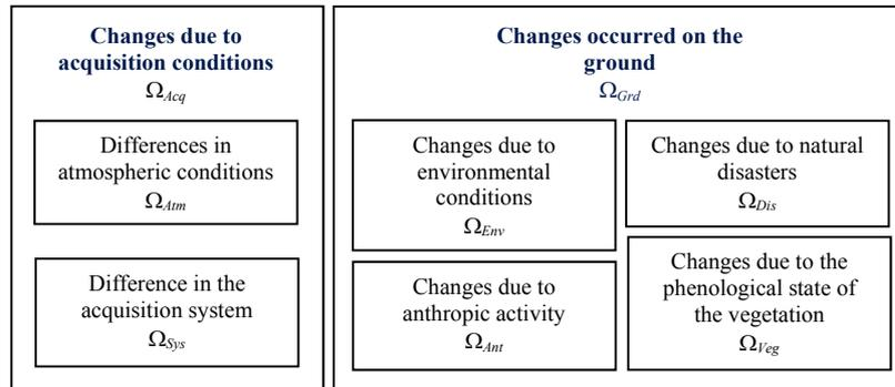
**Figure 3. Taxonomy of the causes of radiometric changes in VHR images.**
