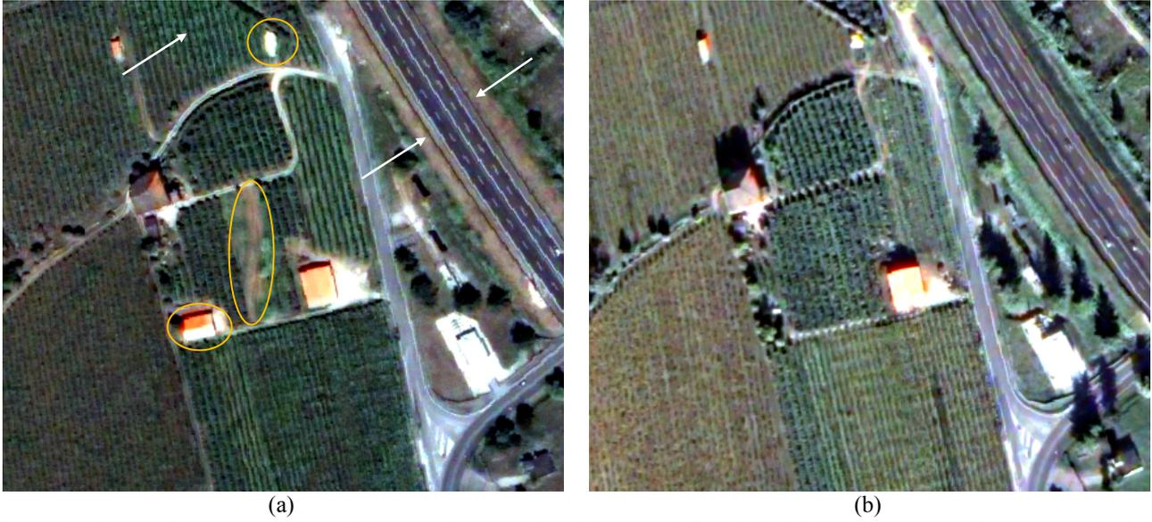
**Figure 11 True color composition of the pansharpener multispectral QuickBird VHR images: (a) image acquired in October 2005; and (b) image acquired in July 2006. Yellow circles and white arrows highlight change locations.**
