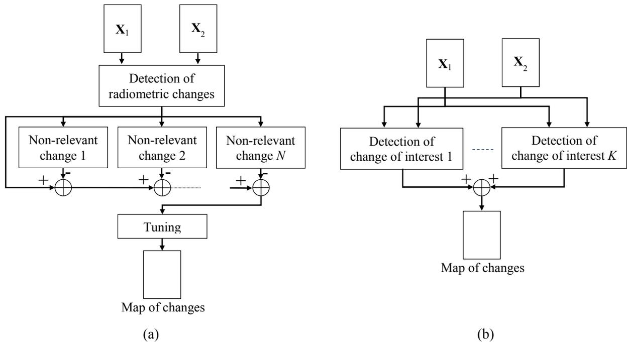
**Figure 7. Proposed architecture based on: (a) differential extraction of changes of interest by cancellation; and (b) direct extraction of changes of interest.**
