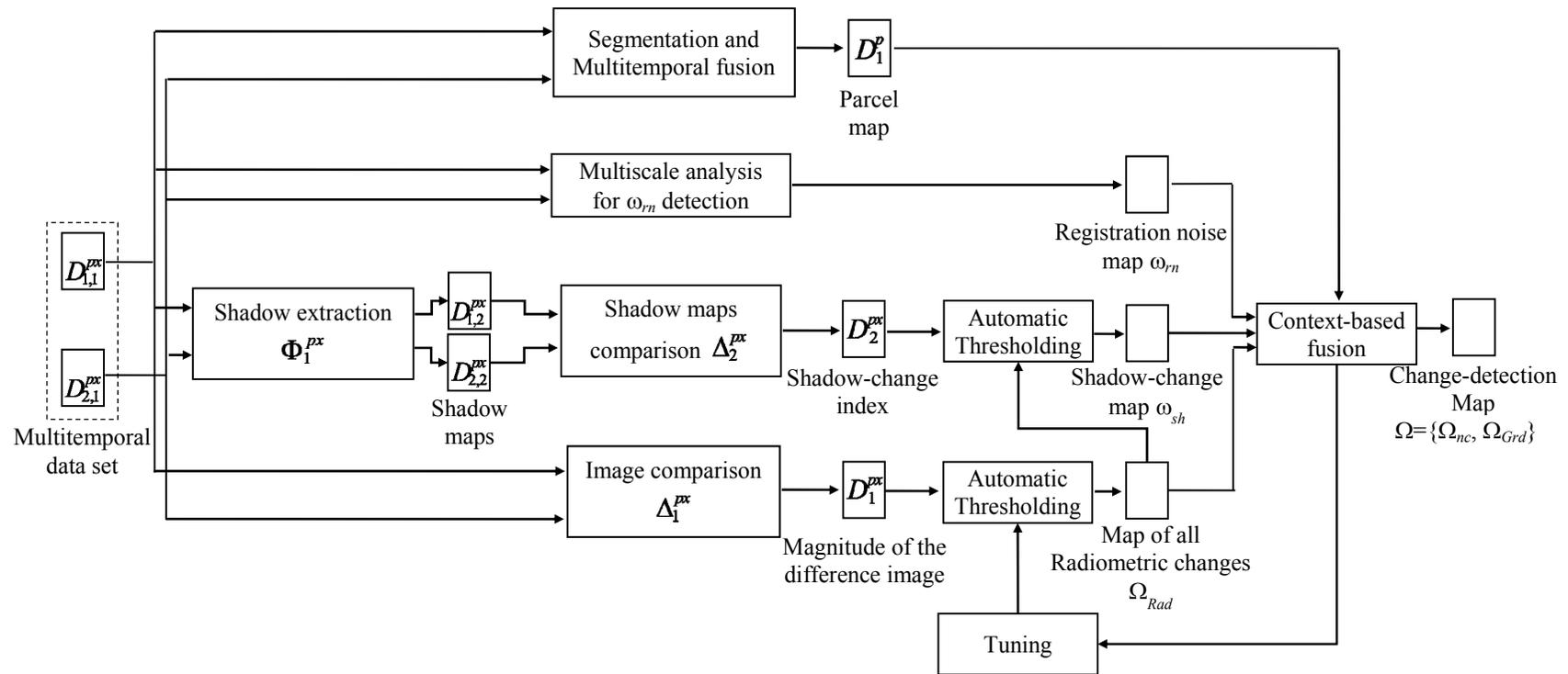
Figure 13. Detailed block scheme of the change detection system defined by using the proposed framework for solving the change-detection problem considered in the example.
