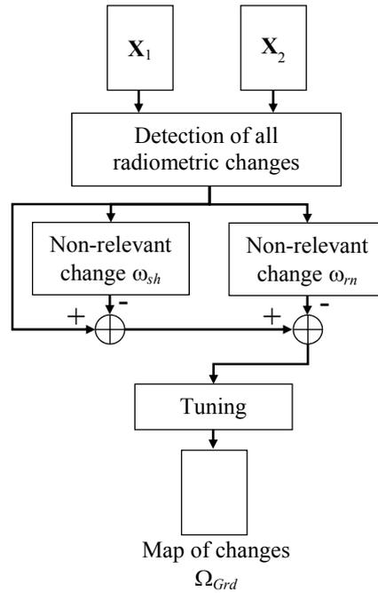
**Figure 12. Block scheme of the general architecture applied for the solution of the considered change-detection problem.**
