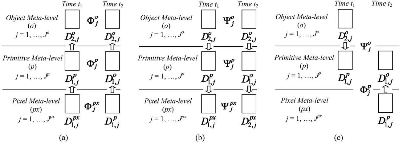
**Figure 9** Schematic representation of the approaches to the multilevel modeling of multitemporal information: (a) simplification (bottom up) approach, (b) prediction (top down) approach, and (c) hybrid approach.
