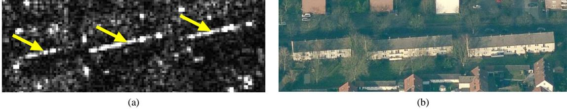
Fig. 5. Examples of gable-roof buildings with large aspect angles. (a) Buildings in 1-meter resolution TerraSAR-X data with viewing direction from left (Infoterra). The scattering lines due to the roofs are highlighted with yellow arrows. (b) The same buildings from (a) in an optical image (Microsoft).
