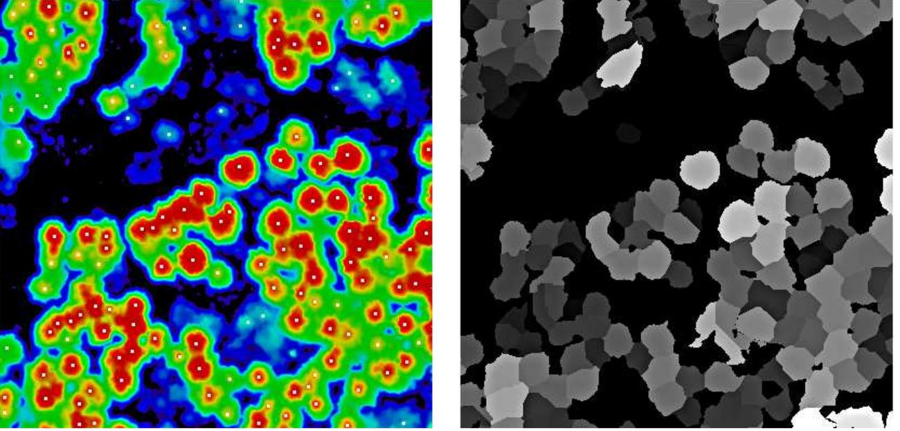
Figure 3. Example of i) seed points extracted from the elevation of the first LIDAR return, and ii) regions associated with the crowns.
