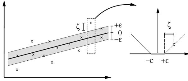
Figure 4.  $\varepsilon$ -insensitive tube of a linear SVR with a linear penalization function (figure source: [34]).
